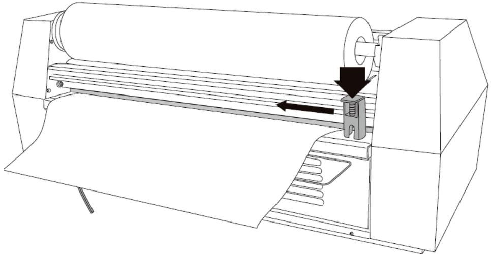
**Caution:** Make sure the cutting edge goes back to the body of the cutter. Otherwise, laminated film will hit the cutter and may cause jamming of film and/or damage of the cutter.
