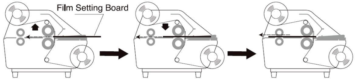
6) Creases (“waterfall”) may appear on the film over the length of the Heat Rollers at the beginning. They will disappear shortly. If they do not disappear, slightly increase the film tension using Tension Controllers on the right sides of the mandrels (rotate them in a clock-wise direction). If both ends of laminated films don't overlap each other properly, adjust the position of the film rolls on the mandrels. If film is not properly overlapped adhesive may get on the rollers.
