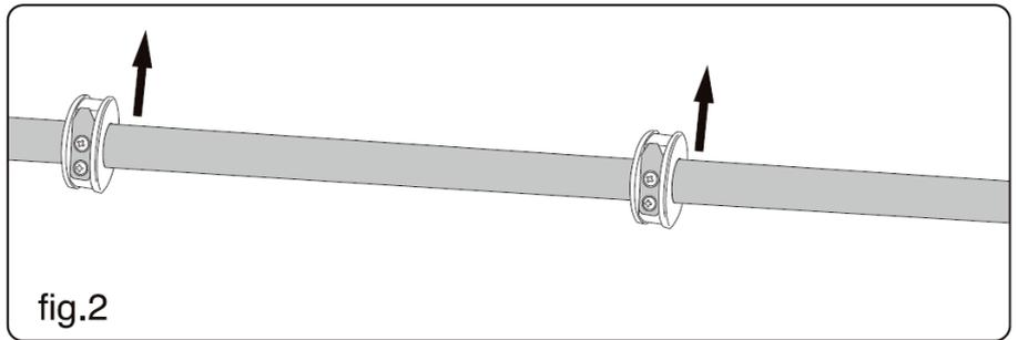
4) Mandrels are preassembled with the mandrel adaptors for a 2-1/4 inch paper core. When you use roll film with a 3 inch paper core, replace the mandrel adaptors accordingly. (fig 3)
