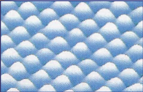
Enlarged representation of a competitor's dimpled adhesive layer surface showing high points and voids.
