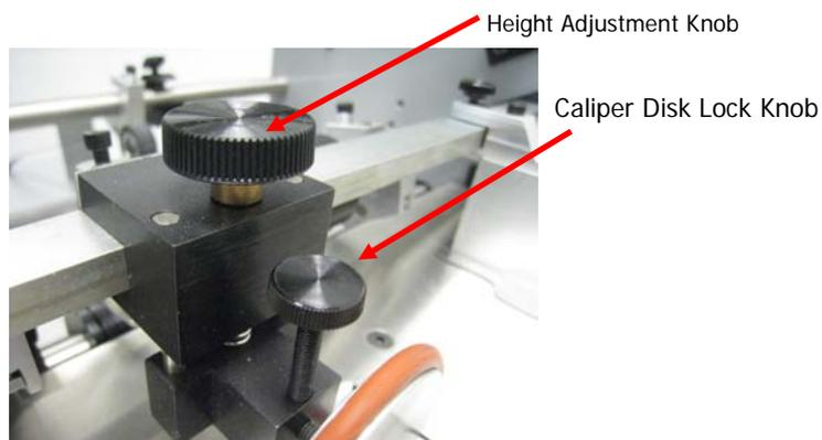
There are 2 different calipers the o-ring and the metal caliper. The metal caliper is designed to work better with heavy stock and the oring caliper is designed to work with lighter stocks. Use the oring caliper when running any multipart forms.
