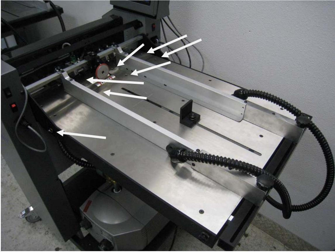
these are the bearing block screws. Also remove the vacuum pickup point adjustment knob from the operator side of the feed table. Now all the lower assemblies will drop to the table. Cut the old orings off the vacuum wheel roll the new orings on the vacuum wheel and reinstall in the reverse order.
