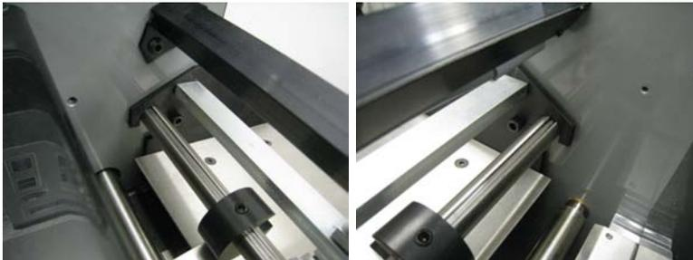
Lift the feed table off and set it on a table. Remove the six flat head screws on the front of the table shown below.
