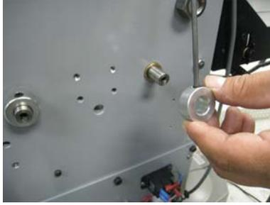
Next, remove the non-operator side cover. Loosen the belt tensioner idler pulley bracket. You do not need to remove these as loosening them will allow enough movement to free the belt. Remove the belt. Walk the motor belt off the inner pulley. If it is too difficult to walk off you could loosen the motor and pull it up as it is mounted in slots.
