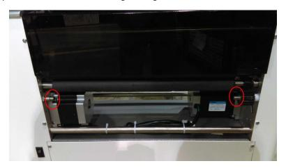
Rest the hooks on the pins above then attach the arms below.
