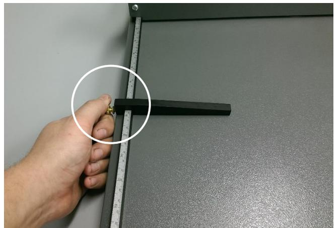
**FIG 2: Position Stops, Tighten Thumbscrews**
