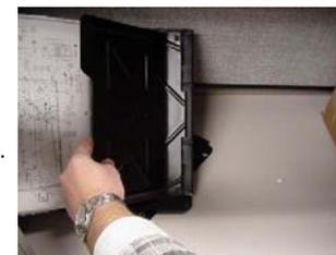
Fold wing to the right until two tabs on the back make contact with the rack.
